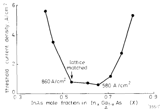
Fig. 1A Threshold current densities against InAs mole fraction x in In x Ga 1-x As quantum wells
